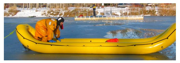
Image 2. The craft surrounds one or more rescuers in an ultra-buoyant and protective inflated perimeter. The RDC allows a rescuer or rescue team to quickly reach a victim and safely retrieve them through the ice or water cold water rescue scene. While on the ice, they are protected from falling through a fracture into the water. In a combination ice and open water situation, the RDC can be paddled across open water or broken ice and water by one or two rescue technicians.
