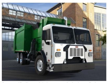
enable an urban refuse truck to operate for up to 65 miles or eight hours on a single charge. It also features a 70 kilowatt onboard battery charger that can fully charge the truck's lithium-ion battery pack in two to four hours.
